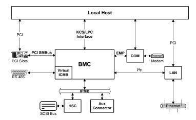
Figure 9. External Interfaces to the BMC
